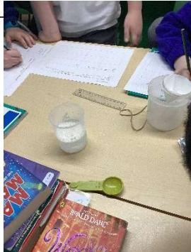
Filtering to separate insoluble solid from liquid.
